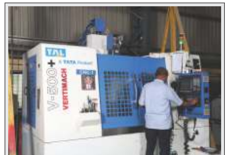
VMC Machine (TAL) 1050 mm x 660 mm x 650 mm
